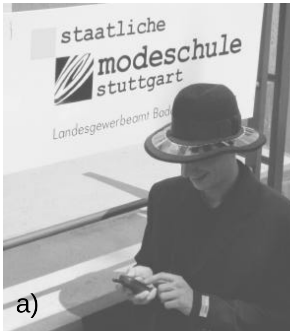
Figure 1: The figures demonstrate the successful construction of the solar hat (figure 1a) and jacket called Jack I (figure 1b) and emphasize the fact, that the integration of photovoltaics onto clothing meets modern fashion design. Monocrystalline silicon is the base material of the solar cells that supply energetically mobile communication electronics such as cellular phones, personal digital assistants (PDAs), MP3 players, radios and world receivers.
