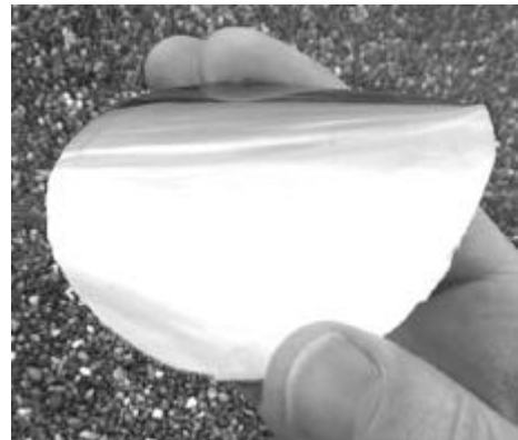
Figure 2: Photograph of a 14 μm thick epitaxial silicon film on top of a 1.5 μm thick QMS film, transferred to a plastic foil.
